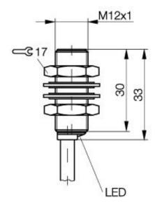
**Inductive Sensors** BES 516-370-E4-C-03 M12x1 x 33 normally-closed Sn=2mm shielded
